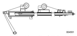
Figure 4-1. Power Mast Cable Routing
