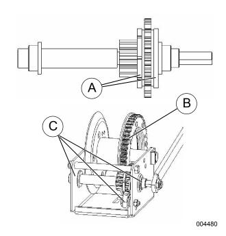
Figure 4-3. Winch Maintenance
