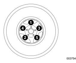
Figure 3-10. Tightening Wheel Lugs
