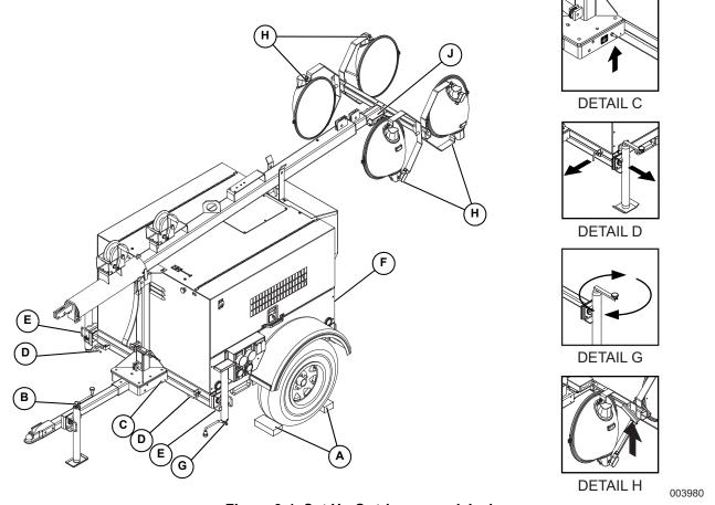
Figure 3-1. Set Up Outriggers and Jacks
