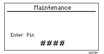
Figure 4-2. Entering Maintenance Pin
